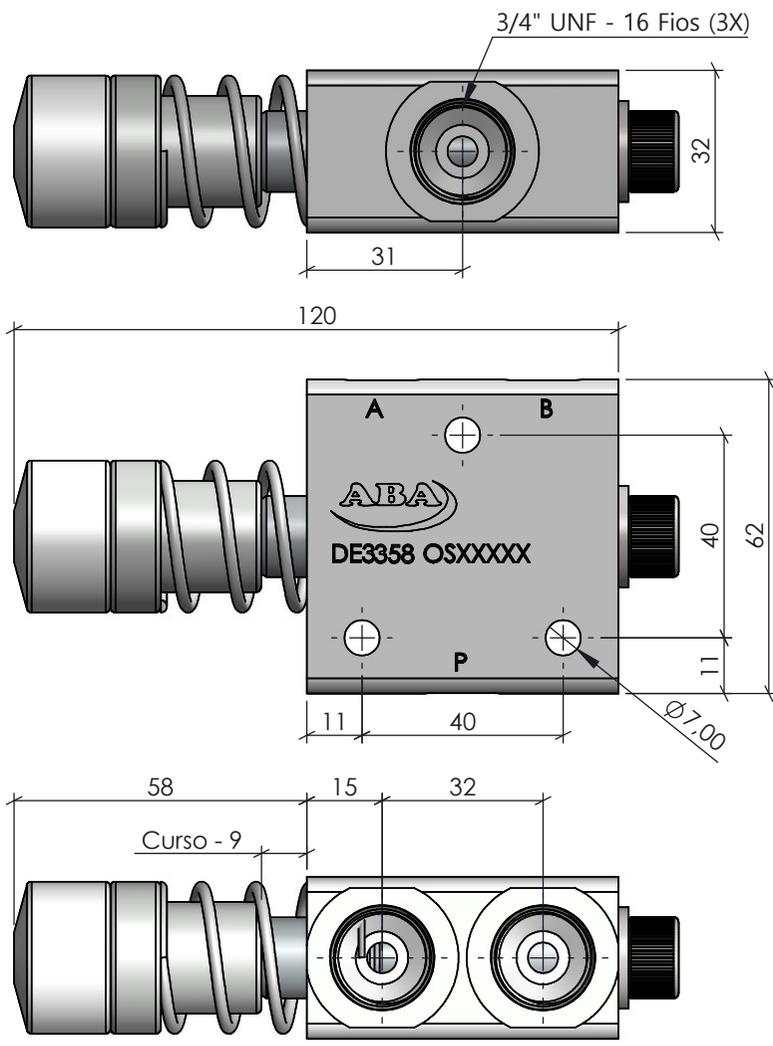
Torque Roscas 3/4" UNF: 35 Nm
