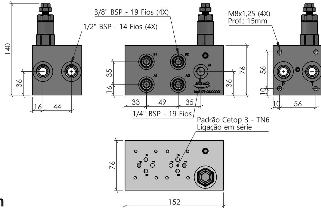
**Torque Roscas 3/8" BSP: 35 Nm**
