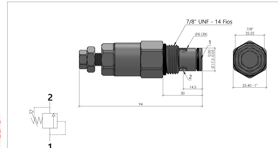
Torque Roscas 7/8" UNF: 50 Nm
